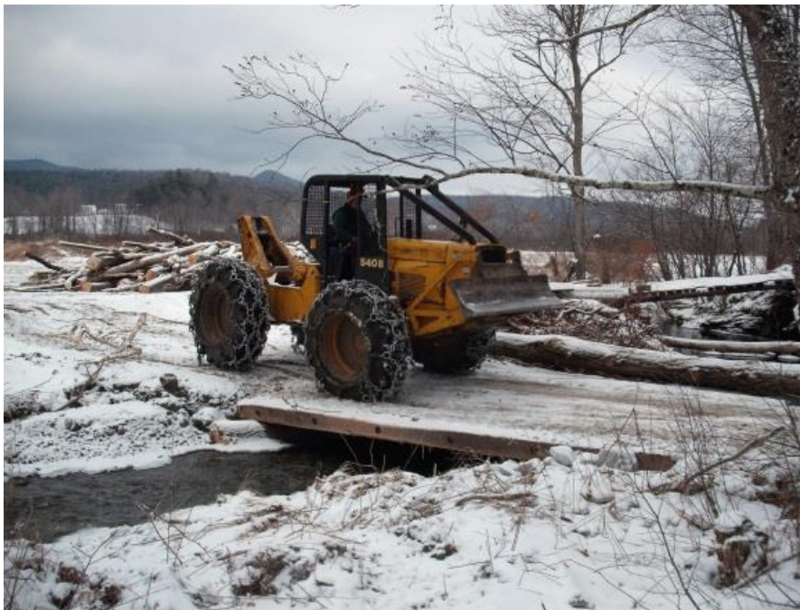
Figure 19. Portable skidder bridges are temporary structures for crossing streams during logging. They are widely accepted as a Best Management Practice for controlling nonpoint source pollution associated with logging operations. When properly utilized, they create less stream bank and stream bed disturbance compared to alternatives such as culverts or log-ford crossings. They are economical as they are reusable, easy to install and can be transported easily.
